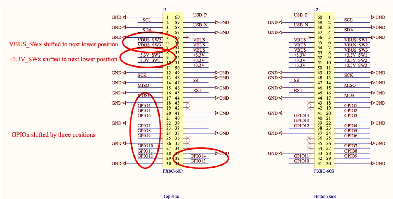
Figure 8: Passthrough connections on a PQ-60 PCB which consumes two power rails and three GPIOs.
