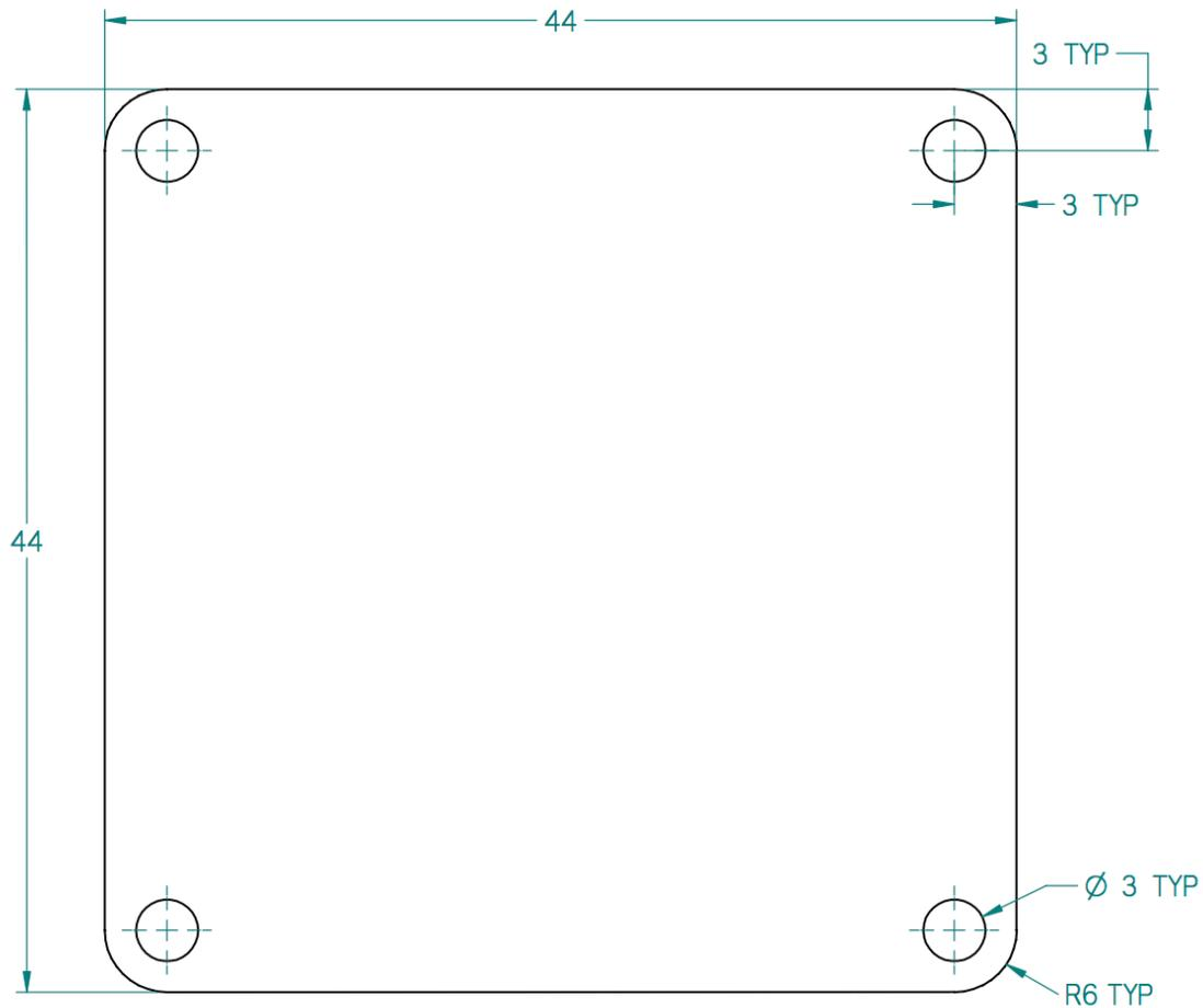
Figure 2: PQ-60 mechanical dimensions.
