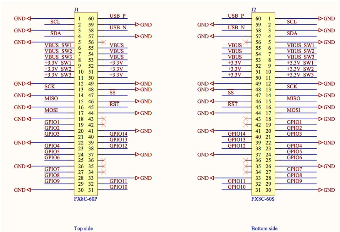
Figure 6: Passthrough connections on a PQ-60 PCB which does not consume any resources.
