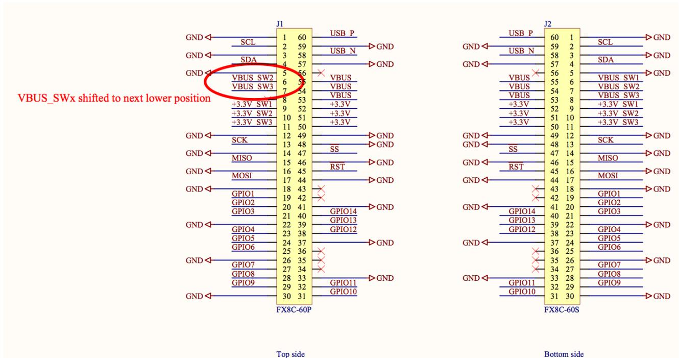
Figure 7: Passthrough connections on a PQ-60 PCB which consumes a single switched power rail.
